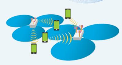
beamforming receiver electronically modifies an antenna pattern to focus the antenna in the direction of an arriving signal. Interfering signals in the direction of the incoming signal are suppressed. modifiable receiver antenna These patterns improve signal quality.
